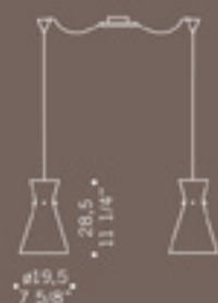
MEMORY S2GD 2x70W E27 alogeno chiara clear halogen 2x75W E27-PAR 30 2x20W E27 fluorescente fluorescent cavo elettrico 200 cm cables length 200 cm
