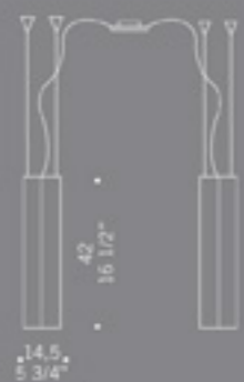
CARRÈ S2GD 2x70W E27 alogeno chiara clear halogen 2x26W E27 fluorescente fluorescent cavo elettrico 200 cm cables length 200 cm
