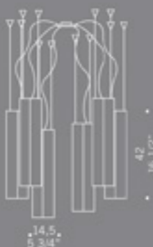
CARRÈ S6GD 6x70W E27 alogeno chiara clear halogen 6x26W E27 fluorescente fluorescent cavo elettrico 200 cm cables length 200 cm
