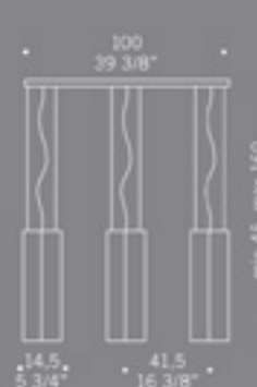
CARRÈ S3PL 3x70W E27 alogeno chiara clear halogen 3x26W E27 fluorescente fluorescent
