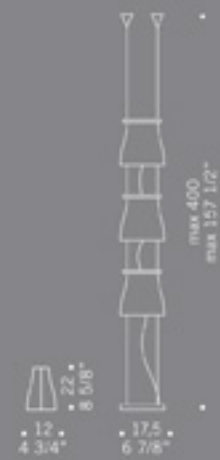
BELL S3V 3x60W G9 alogeno bispina halogen bi-pin con varialuce with dimmer
