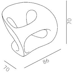
Hara is a bio-energetic seat handmade in lacquered fibreglass. Ideal for outdoors thanks to a treatment against ultra-violet rays and to the strong resistance of the material to temperature changes.
